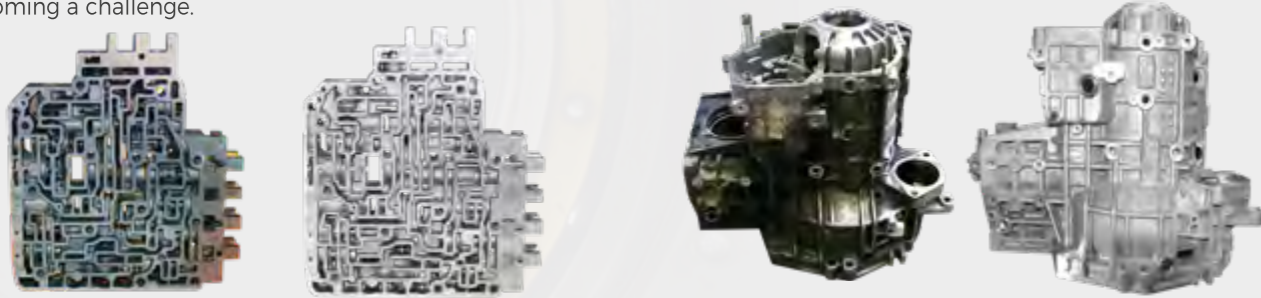
BEFORE AND AFTER. CLEANING OF VALVE BOX AND GEARBOX
